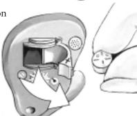
Step 3: Swing the door into the closed position. The compartment should close easily. Do not force it. If resistance is noted, check that the battery is inserted correctly.
